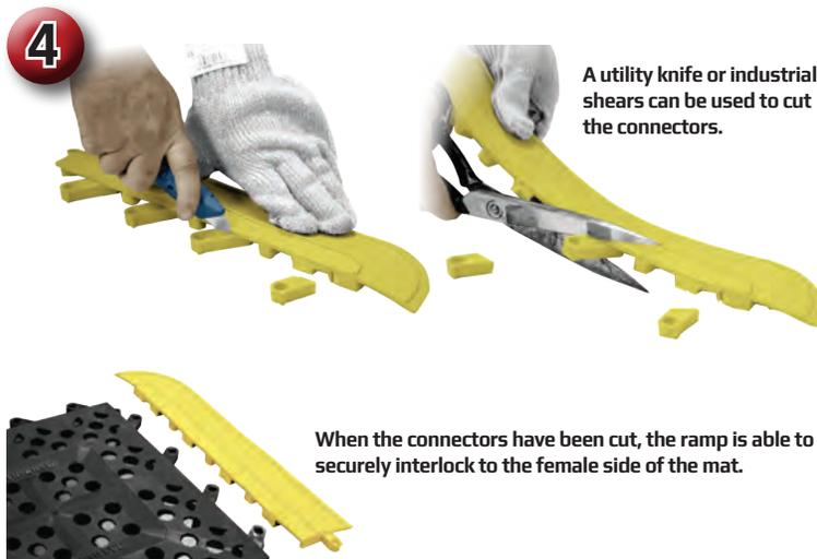
A utility knife or industrial shears can be used to cut the connectors.
