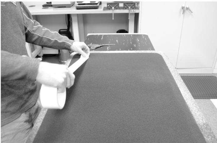
2. Cut tape and press along the strip to ensure it is firmly applied.
