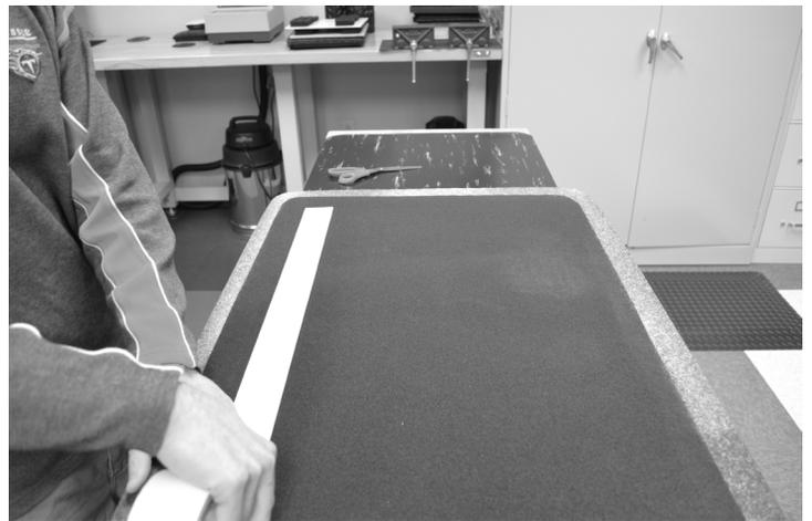
3. Peel off the white top layer leaving the clear tape behind.
