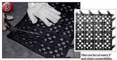
Use a utility knife or sharp shears to cut tiles.
